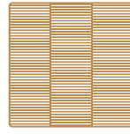
Backed strips for mosaic laying
